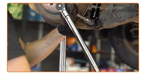
Tighten the lower fastener of the shock absorber. Use a drive socket #E20. Use a torque wrench. Tighten it to 72 Nm torque.
