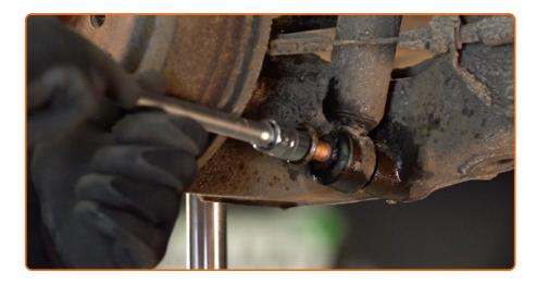
Unscrew the lower fastener of the shock absorber. Use a drive socket #E20. Use a tap wrench.
