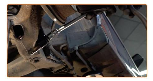
Screw in the lower fastener of the shock absorber. Use a drive socket #E20.
