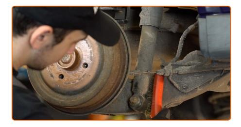
Clean the shock absorber fasteners.
