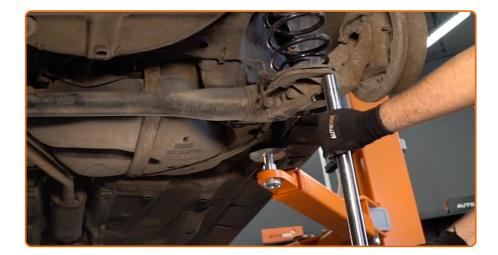
Remove the support from under the arm.
