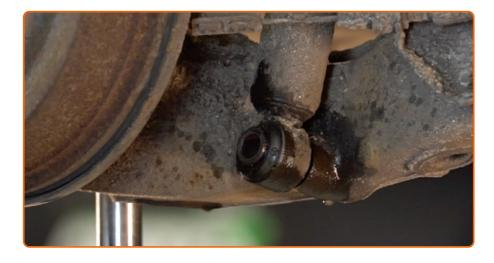
Remove the fastening bolt.
