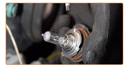
Remove the old bulb. Use a flat screwdriver.
