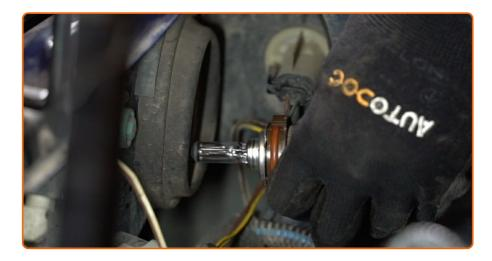
Install the bulb holder into the headlight mounting seat. Secure the bulb holder by turning it by  $^{\sim}30^{\circ}$ .
