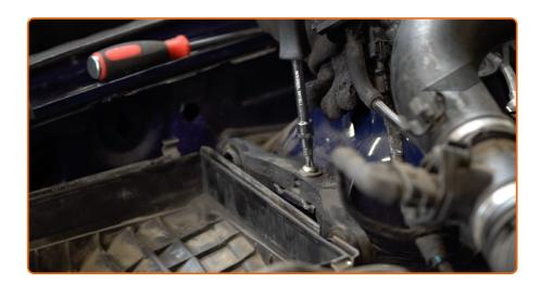
Screw the filter housing fastening bolts. Use Torx T30. Use a ratchet wrench.
