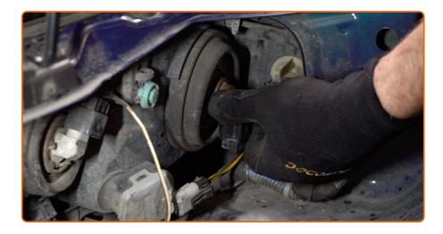
Detach the bulb holder by turning it by  $^{\sim}30^{\circ}$ . Remove the holder from the headlight mounting seat.
