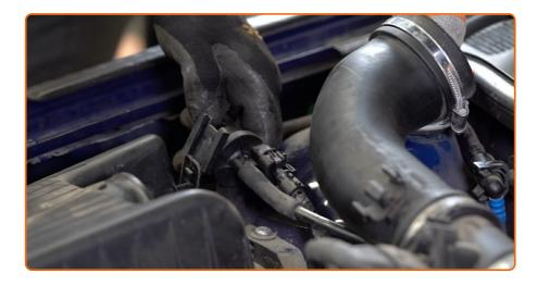
Detach the fasteners connecting the air pipe and the wiring harness to the air filter housing.
