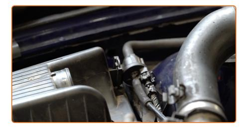
Attach the fasteners connecting the air pipe and the wiring harness to the air filter housing.
