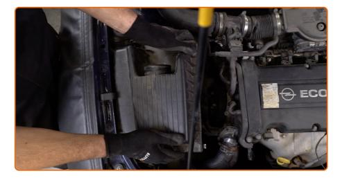
Take off the filter lid. Remove the filter element from the filter housing.
