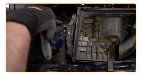
Unscrew the filter housing fastening bolts. Use Torx T30. Use a ratchet wrench.
