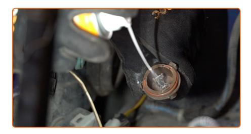
Clean the bulb mounting seat on the holder. Use electronic spray.
