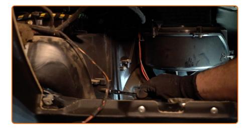
Unscrew the fasteners of the cabin filter housing cover. Use a drive socket #7.
