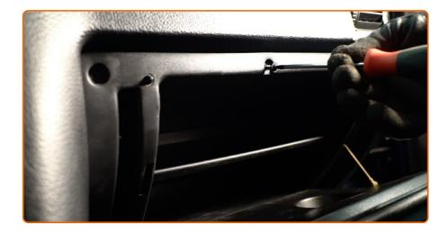
Unscrew the glove box fastening screws. Use Torx T20.
