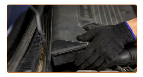
Reinstall the air filter housing.
