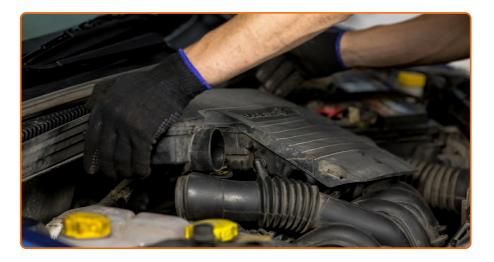
Remove the air filter housing.
