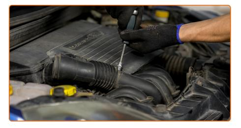
Remove the crankcase ventilation hose. Use a flat screwdriver.
