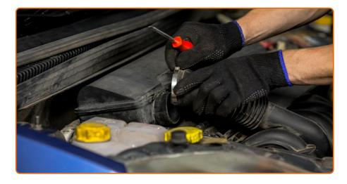
Detach the air intake hose clamp. Use a flat screwdriver.
