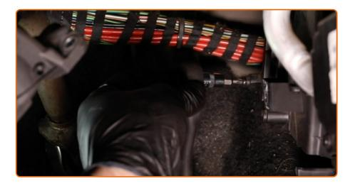
Unscrew the fasteners of the cabin filter housing cover. Use Torx T20. Use a ratchet wrench.
