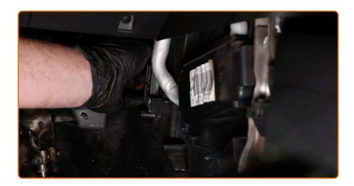
Reinstall the cabin filter housing cover.
