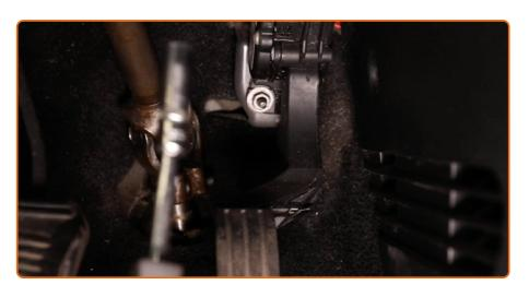
Unscrew the fastener of the accelerator pedal and move it aside. Use a drive socket #10. Use a ratchet wrench.
