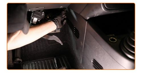
Reinstall the clips of the plastic side panel.
