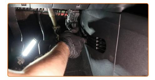
Return the accelerator pedal to its initial position and screw in its fastener. Use a drive socket #10. Use a ratchet wrench.
