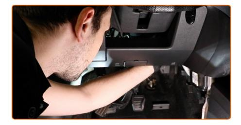
Screw in the fasteners of the cabin filter housing cover. Use Torx T20. Use a ratchet wrench.
