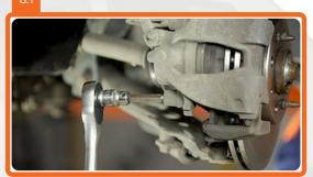
Unscrew the brake caliper fastening
