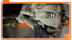
With a simple screwdriver remove caps from both guide pins.
