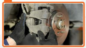
Install the brake caliper and fix it.
