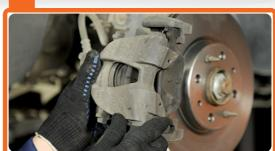
Remove the brake caliper.
