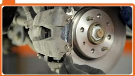
Install the brake caliper spring
