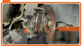
Remove the brake pads.
