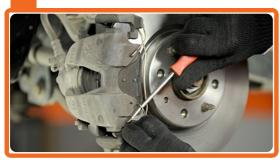
Using a simple screwdriver, remove the brake caliper spring clip.
