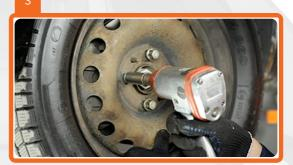
Loosen the wheel mounting bolts.
