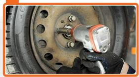
Lower the car and working in a cross order, tighten the wheel bolts.
