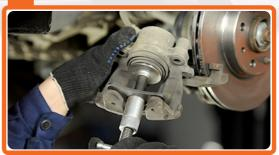
With the help of a special tool push in the brake caliper piston to a stop.
