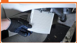
Install a new cabin filter according to the mark.
