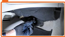
Remove the protective cover under the glove box.
