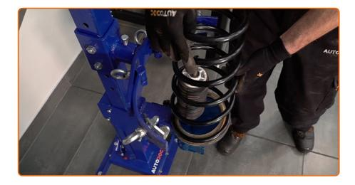
Install the spring on the shock absorber.
