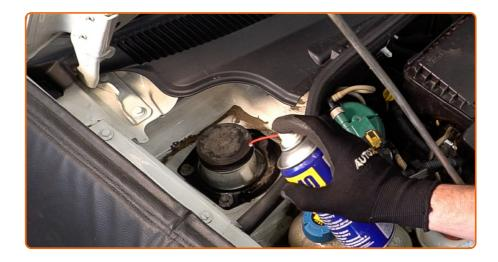
Clean the fasteners of the shock strut upper mount. Use WD-40 spray.
