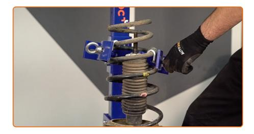
Release the coil spring.
