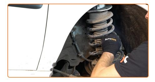
Remove the suspension strut.
