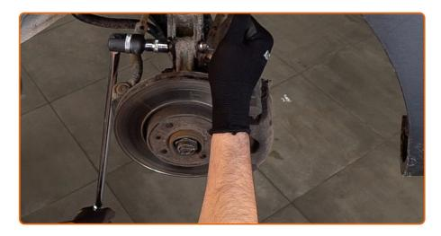
Unscrew the lower fastener connecting the shock strut to the steering knuckle. Use a combination spanner #19. Use a drive socket #19. Use a tap wrench.
