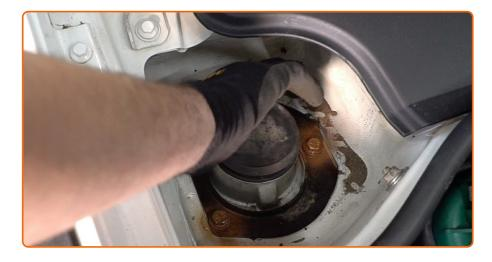
Install the shock strut mount cap.
