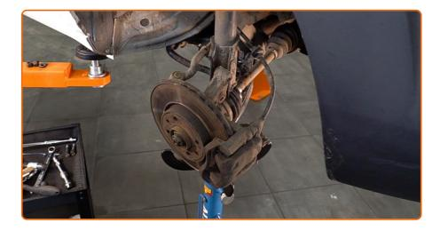
Disconnect the steering knuckle from the shock absorber strut. Use a pin punch. Use a rubber mallet.
