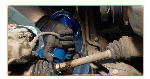
Fasten the brake hose on the strut.
