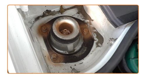
Treat the fasteners of the shock strut mount. Use copper grease.
