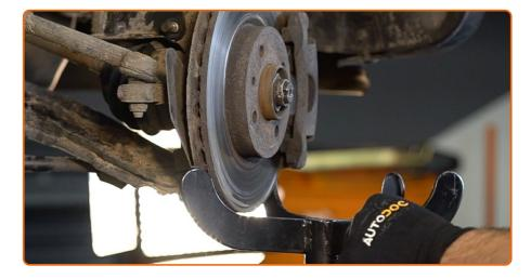
Prop up the steering knuckle. Use a hydraulic transmission jack.
