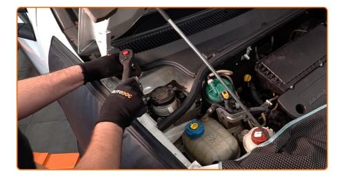
Loosen the upper fastener of the shock strut mount. Use a drive socket #13. Use a ratchet wrench.
