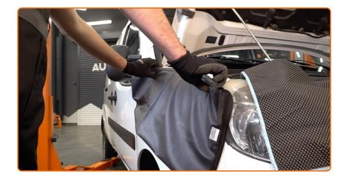
Remove the fender protection cover.
