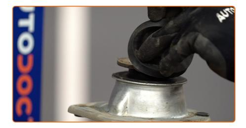
Remove the shock strut mount cap.
