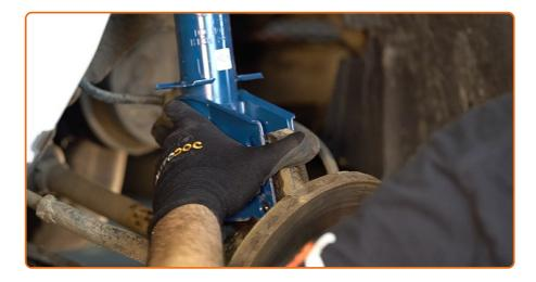
Fix the shock absorber strut on the steering knuckle. Use a crowbar.
