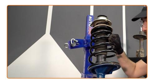
Remove the assembled shock strut.
