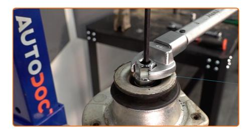
Tighten the shock strut piston rod nut. Use a drive socket #19. Use HEX No.H6. Use a torque wrench. Tighten it to 60 Nm torque.
