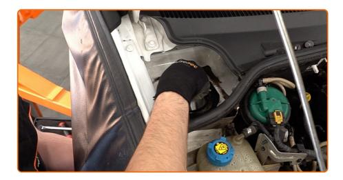
Unscrew the top fastening of the shock strut mount.
