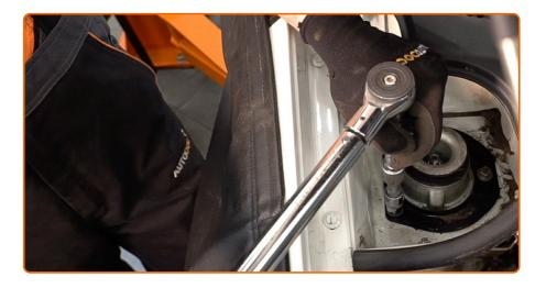
Tighten the upper fastener of the shock absorber strut mount. Use a drive socket #13. Use a torque wrench. Tighten it to 32 Nm torque.
