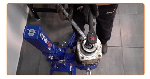
Remove the strut piston rod nut. Use a drive socket #19. Use HEX No.H6.
