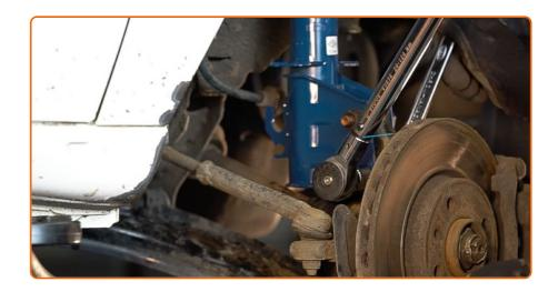
Tighten the lower fasteners connecting the shock strut to the steering knuckle. Use a drive socket #19. Use a combination spanner #19. Use a torque wrench. Tighten it to 83 Nm torque.
