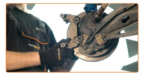
Remove the caliper bracket.
