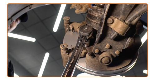
Tighten the brake caliper bracket. Use a drive socket #19. Use a torque wrench. Tighten it to 68 Nm torque.
