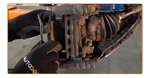
Remove the brake pads. Use a crowbar.
