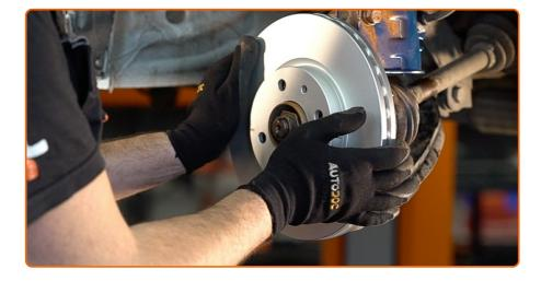
Install the brake disc.
