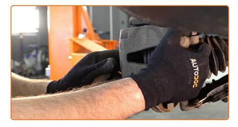
Remove the brake caliper.
