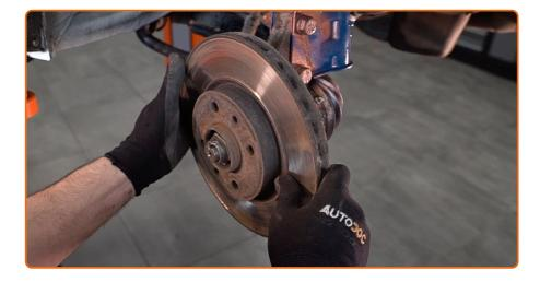
Remove the brake disc.
