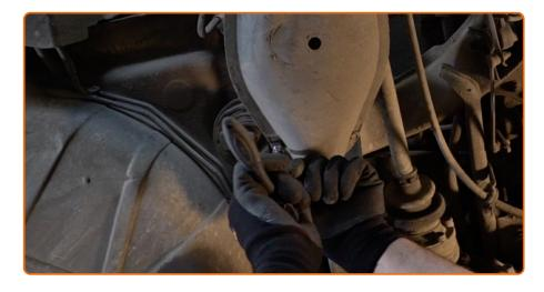
Unscrew the fasteners of the control arm plastic cover. Use a drive socket #10. Use a ratchet wrench.
