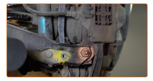
Align the fastener holes of the stabilizer link and the suspension control arm. Use a pin punch. Use a rubber mallet.
