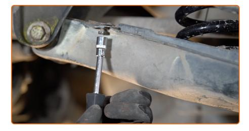
Screw the fasteners of the control arm plastic cover. Use a drive socket #10. Use a ratchet wrench.
