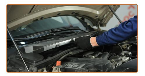
Reinstall the cabin filter housing cover.
