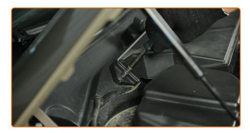
Screw in the fasteners of the cabin filter housing cover (6 pieces). Use a drive socket #8. Use a ratchet wrench.
