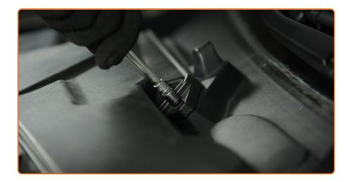
Unscrew the fasteners of the cabin filter housing cover (6 pieces).
