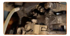
Tighten the brake bleeder screw. Use a drive socket #11. Use a ratchet wrench.
