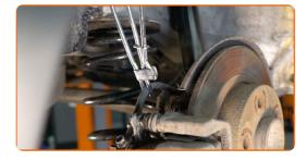
Unscrew the brake hose from the brake caliper. Use a combination spanner #11.
