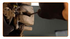
Remove the brake caliper. Use a crowbar.
