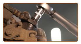
Remove the brake hose clamp.
