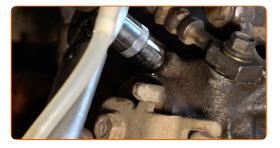
Tighten the brake caliper bleed screw. Use a drive socket #11. Use a torque wrench. Tighten it to 10 Nm torque.
