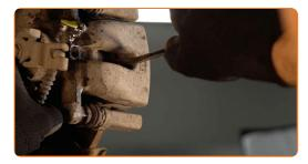
Remove the brake caliper. Use a crowbar.
