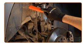
Unscrew the nut and remove the stabilizer rod from the shock strut. Use a combination spanner #19. Use a drive socket #19. Use a ratchet wrench.
