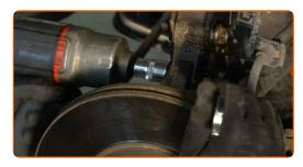
Clean the fasteners of the ABS sensor and of the brake hose which connect them to the shock strut. Use a wire brush. Use WD-40 spray.
