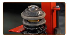
Tighten the shock strut piston rod nut. Use HEX No.H6. Use a drive socket #22. Use a torque wrench. Tighten it to 65 Nm torque.
