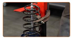
Install the mount, the boot and the bump stop on the shock absorber.
