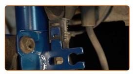
Fasten the brake hose on the strut. Use a rubber mallet.
