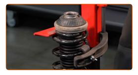
Remove the assembled shock strut.
