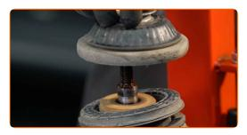
Release the coil spring.
