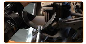
Install the retainer of the shock strut upper mount. Use water pump pliers.
