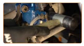
Tighten the lower fasteners connecting the shock strut to the steering knuckle. Use a combination spanner #18. Use a drive socket #18. Use a torque wrench. Tighten it to 105 Nm torque.
