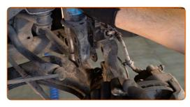
Remove the retainer of the shock strut upper mount.
