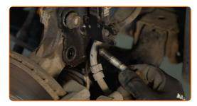
Disconnect the steering knuckle from the shock absorber strut. Use a crowbar.
