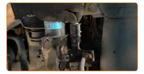
Detach the brake hose from the shock strut. Use water pump pliers.
