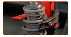
Remove the strut piston rod nut. Use HEX No.H6. Use a drive socket #22. Use a ratchet wrench.
