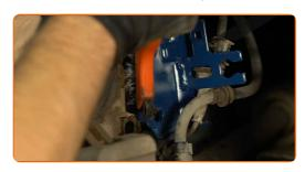
Fix the shock absorber strut on the steering knuckle.
