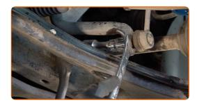
Unscrew the fastener connecting the stabilizer link to the shock strut. Use a combination spanner #19. Use a drive socket #19. Use a ratchet wrench.
