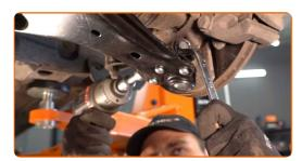
Tighten the ball joint fastener. Use a drive socket #19. Use a combination spanner #17. Use a torque wrench. Tighten it to 50 Nm torque.
