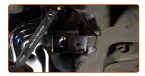
Tighten the rear fastener of the control arm. Use a combination spanner #18. Use a drive socket #18. Use a torque wrench. Tighten it to 90 Nm torque.+90°
