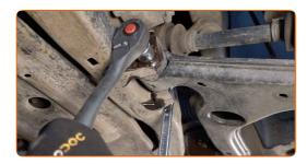
Loosen the rear fastener of the control arm. Use a drive socket #18. Use a combination spanner #18. Use a ratchet wrench.
