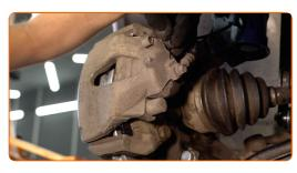
51 Snap the brake caliper retaining spring back into place. Use a crowbar.
