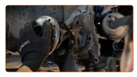
Clean the hub bearing mounting seat. Use a wire brush. Use WD-40 spray.
