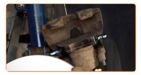
Install the brake caliper and fix it.
