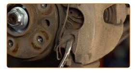
11 Remove the brake caliper.
