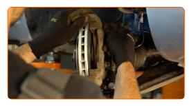
Tighten the brake caliper bracket. Use a drive socket #18. Use a torque wrench. Tighten it to 100 Nm torque.
