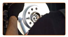
Install the brake caliper bracket.
