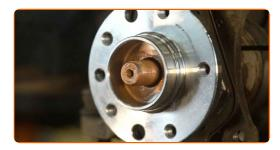
Screw the wheel hub axle nut. Use a drive socket #32.
