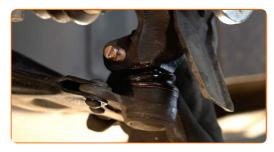
Tighten the ball joint fastener. Use a combination spanner #17. Use a drive socket #19. Use a torque wrench. Tighten it to 50 Nm torque.
