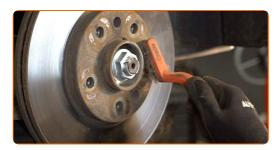
Unscrew the brake disc fastening. Use HEX No.H5. Use a ratchet wrench.
