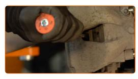
Pull aside the brake caliper retaining spring. Use a crowbar.
