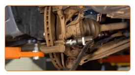
Remove the caliper bracket.
