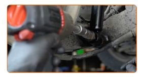
9 Remove the fastening bolt.
