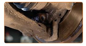
Unscrew the front arm fastener. Use a combination spanner #18. Use a drive socket #18. Use a ratchet wrench.
