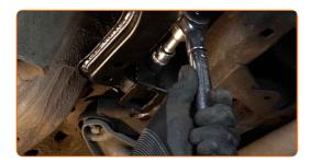
Tighten the front fastener connecting the control arm to the subframe. Use a drive socket #18. Use a torque wrench. Tighten it to 100 Nm torque.
