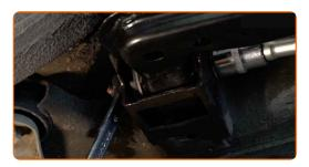
Tighten the rear fastener connecting the arm to the body subframe. Use a drive socket #18. Use a torque wrench. Tighten it to 100 Nm torque.
