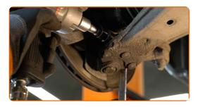
Remove the fastening bolt.
