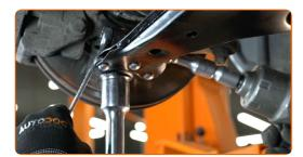
Screw the front arm fastener. Use a combination spanner #18. Use a drive socket #18. Use a tap wrench.
