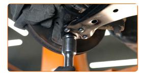
Screw the fasteners of the ball joint. Use a combination spanner #18. Use a drive socket #18. Use a ratchet wrench.
