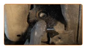
Release the fastener that connects the control arm ball joint to the steering knuckle. Use a flat metal-working chisel. Use a hammer.
