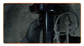
Tighten the stabiliser link fastener. Use a combination spanner #19. Use a drive socket #19. Use a ratchet wrench.
