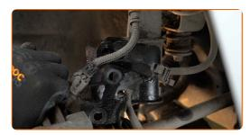
27 Unscrew the top fastening of the shock strut mount.
