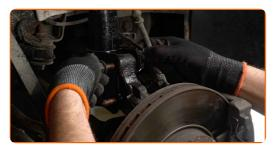
Screw in the fastener that connects the shock strut to the steering knuckle. Use a combination spanner #18. Use a drive socket #18. Use a ratchet wrench.
