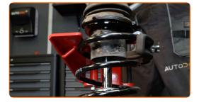
Remove the assembled shock strut.
