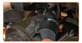
Clean the fasteners connecting the brake hose to the shock strut. Use a wire brush. Use WD-40 spray.
