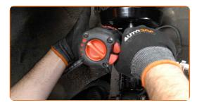
Tighten the fastener connecting the stabilizer link to the shock strut. Use a drive socket #19. Use a torque wrench. Tighten it to 60 Nm torque.
