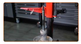
Install the spring on the shock absorber.
