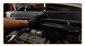
Clean the fasteners of the lower part of the scuttle panel. Use WD-40 spray.
