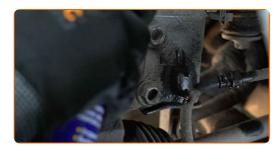
Unscrew the lower fastener connecting the shock strut to the steering knuckle. Use a combination spanner #18. Use a drive socket #18. Use a tap wrench.
