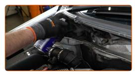
Loosen the upper fastener of the shock strut mount. Use a combination spanner #18. Use HEX No.H6. Use a ratchet wrench.
