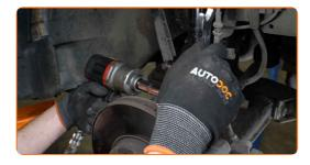
Tighten the lower fasteners connecting the shock strut to the steering knuckle. Use a combination spanner #18. Use a drive socket #18. Use a torque wrench. Tighten it to 90 Nm torque.+45°
