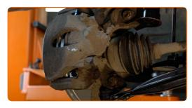
20 Install the brake caliper retaining spring.
