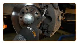
11 Remove the brake caliper.
