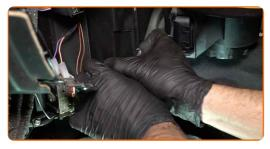
Reinstall the air distribution housing assembly.
