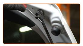
Release the circlip connecting the gas strut to the car body. Use a flat screwdriver.
