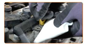
Move the wiring harness bracket aside.
