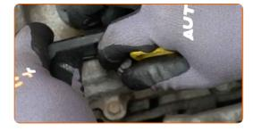
Tighten the fasteners of the wiring harness bracket. Use a drive socket #10. Use a torque wrench. Tighten it to 9 Nm torque.
