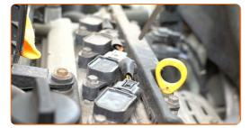
Unscrew the fasteners of the wiring harness bracket. Use a drive socket #10. Use a ratchet wrench.
