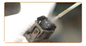
Attach the ABS sensor connector.
