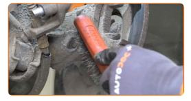
Unscrew the brake caliper bracket fasteners. Use a drive socket #14. Use a ratchet wrench.
