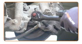
Remove the brake caliper. Use a crowbar.
