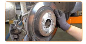
Clean the ABS sensor fastener. Use a nylon cleaning brush. Use all-purpose cleaning spray.
