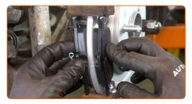
Install the brake caliper and fix it.
