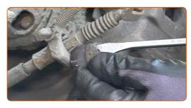
Unscrew the brake caliper fasteners. Use HEX No.H7. Use a ratchet wrench.
