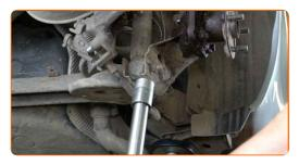
Unscrew the wheel hub bearing fasteners. Use a drive socket #14. Use a ratchet wrench.
