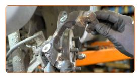
16 Remove the brake disc.
