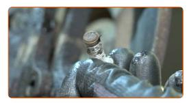
Remove the caliper bracket.
