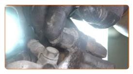
Install the brake caliper retaining spring.
