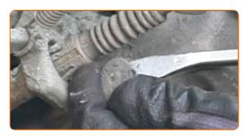
Unscrew the brake caliper fasteners. Use HEX No.H7. Use a ratchet wrench.
