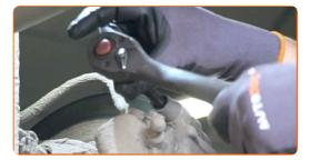
Remove the brake caliper. Use a crowbar.
