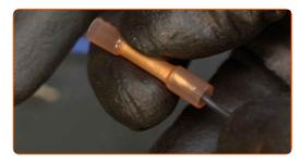
Crimp the solder sleeves. Use crimping pliers.
