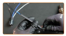
Using solder sleeves, splice the oxygen sensor wires with the connector wires according to the colour coding.
