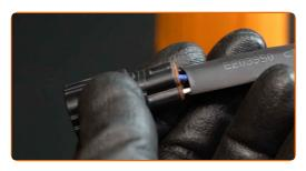
Shrink the heat shrink tube. Use a heat gun.
