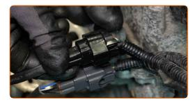
Fasten the oxygen sensor wiring with the clamp.
