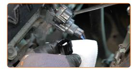
Attach the oxygen sensor connector.
