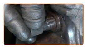
Clean the oxygen sensor mounting seat. Use all-purpose cleaning spray.
