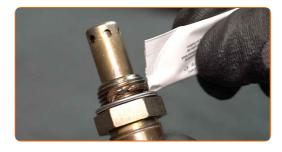
21 Install the new oxygen sensor.
