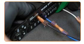
Shrink the heat shrink tubes of the solder sleeves. Use a heat gun.
