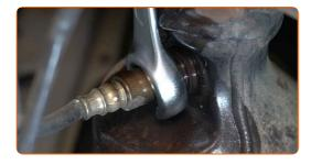
7 Remove the oxygen sensor.
