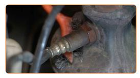
Unscrew the oxygen sensor fastener. Use a flare nut spanner #22. Use a ratchet wrench.
