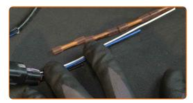
Shorten the wires of the new oxygen sensor in a corresponding way. Use nippers.
