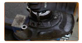
Install the wheel hub on the steering knuckle. Use a bush and bearing driver set.
