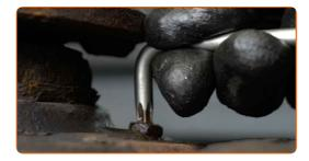
Remove the hub from the steering knuckle. Use a bush and bearing driver set.
