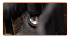
Tighten the fastener that connects the ABS sensor to the steering knuckle. Use a drive socket #10. Use a torque wrench. Tighten it to 8 Nm torque.
