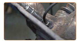
Tighten the lower fasteners connecting the shock strut to the steering knuckle. Use a combination spanner #19. Use a drive socket #19. Use a torque wrench. Tighten it to 164 Nm torque.
