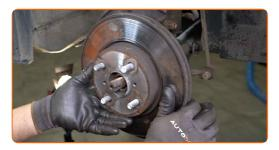
70 Install the brake caliper together with its bracket.
