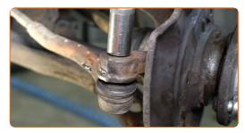
Install the cotter pin that secures the fastener connecting the tie rod end to the steering knuckle. Use a crowbar.
