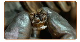
Disconnect the ball joint from the steering knuckle. Use a ball joint puller.
