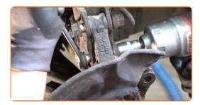
Screw the fastener connecting the ball joint to the steering knuckle. Use a combination spanner #19.
