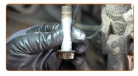
Detach the driveshaft from the steering knuckle.
