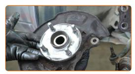
Clean the mounting seats of the shock strut. Clean the splines of the drive shaft CV joint. Clean the fastener connecting the ball joint to the steering knuckle. Clean the fastener connecting the tie rod end to the steering knuckle. Use a wire brush. Use WD-40 spray.
