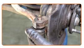
Tighten the fastening nut connecting the tie rod end to the steering knuckle. Use a drive socket #17. Use a torque wrench. Tighten it to 49 Nm torque.
