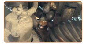
Tighten the brake caliper bracket fasteners. Use a drive socket #17. Use a torque wrench. Tighten it to 107 nm torque.
