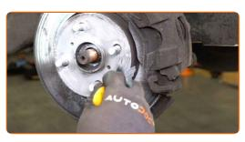
75 Clean the brake disk surface. Use a brake cleaner.
