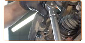
Install the dust boot caps of the brake caliper guide pins.
