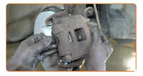
Tighten the brake caliper fasteners. Use HEX No.H7. Use a torque wrench. Tighten it to 34 nm torque.
