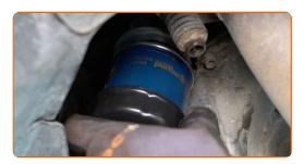
Tighten the oil filter. Remember to observe the recommended tightening torque. Use the 65-14F socket. Use a torque wrench. Tighten it to 24 Nm torque.
