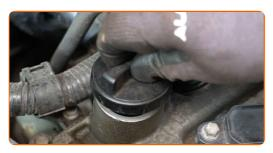
Tighten the oil filler cap.
