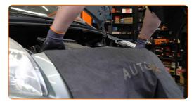
Release the air filter cover clips.
