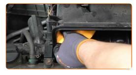
Remove the filter element from the air filter cover.
