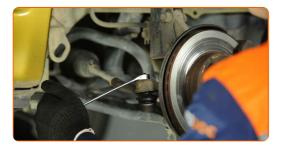
Install the cotter pin fixing the tie rod end fastening. Use nippers.
