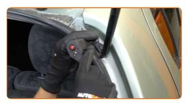
Unscrew the fastener connecting the gas strut to the boot lid. Use a drive socket #10. Use a ratchet wrench.
