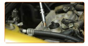
Screw new spark plugs and tighten them. Use the spark plug socket #16. Use a torque wrench. Tighten it to 22 nm torque.
