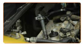
Tighten the fasteners of the ignition coils. Use a drive socket #10. Use a ratchet wrench.
