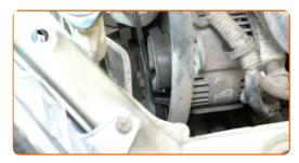
Loosen the tensioner lever of the V-ribbed belt. Use a combination spanner #12.
