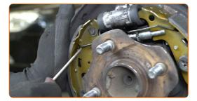
Install the lower return spring. Use a flat screwdriver.
