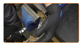
Remove the brake shoe hold-down cup.
