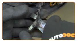
Perform further demounting of the upper retaining spring and the adjuster mechanism.
