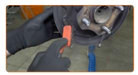
Loosen the vice and remove the brake shoes.
