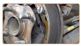
Move the parking brake shoes against the drum. Use a crowbar. Use a flat screwdriver.
