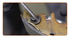
Remove the brake shoe adjuster lever. Use a flat screwdriver.
