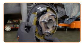
Reinstall the brake shoe hold-down pin. Use a brake shoe retaining spring compressor.
