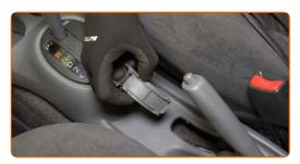
Loosen the parking brake cable. Use a drive socket #10. Use a ratchet wrench.
