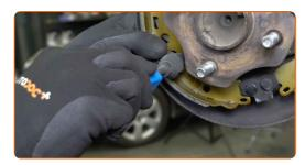
Install the upper return spring. Use a flat screwdriver.
