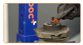
Remove the strut piston rod nut. Use a drive socket #17. Use a ratchet wrench.
