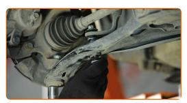
Use a combination spanner #13. Use a drive socket #13. Use a torque wrench. Tighten it to 18 Nm torque.
