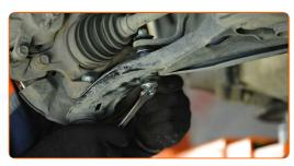
Treat all joints of the stabiliser link. Use copper grease.
