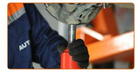
Tighten the fastener connecting the stabilizer link to the stabilizer bar. Use a combination spanner #13. Use a drive socket #13. Use a torque wrench. Tighten it to 18 Nm torque.
