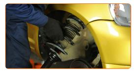
Screw the top fastening of the shock strut mount.
