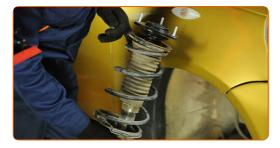
Set the shock absorber strut on the spring compressor tool.
