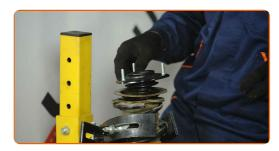
Tighten the shock strut piston rod nut. Use a drive socket #17. Use a torque wrench. Tighten it to 33 Nm torque.
