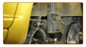
Remove the bracket from the shock absorber strut.
