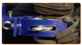
Remove the protective cap from the shock absorber strut mount. Use a flat screwdriver.
