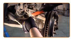
Unscrew the lower fastener connecting the shock strut to the steering knuckle. Use a combination spanner #19. Use a drive socket #19. Use a ratchet wrench.
