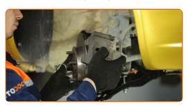
Tighten the brake caliper bracket. Use a drive socket #17. Use a torque wrench. Tighten it to 88 Nm torque.
