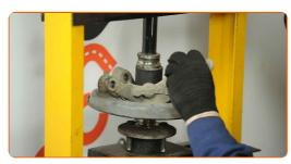
Install the steering knuckle with a hub in assembly.
