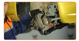
Remove the steering knuckle together with the hub.
