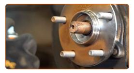
45 Install the brake disc.
