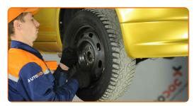
6 Unstake the fastener of the driveshaft. Use a flat metal-working chisel. Use a hammer.
