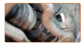
Tighten the drive shaft nut. Use a drive socket #30. Use a tap wrench. Use a torque wrench. Tighten it to 216 Nm torque.
