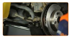
Tighten the fastening nut connecting the tie rod end to the steering knuckle. Use a combination spanner #17. Use a torque wrench. Tighten it to 49 nm torque.
