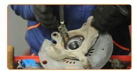
Press the wheel hub into the bearing inner race. Use a bush and bearing driver set.
