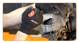
Unscrew the brake caliper fastening. Use a combination spanner #17. Use a drive socket #14.
