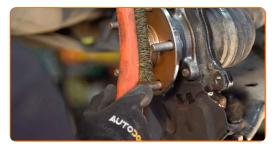
17 Install the brake disc.
