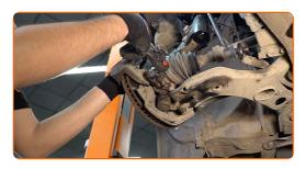
Remove the caliper bracket.
