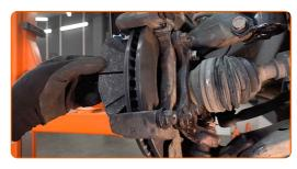
Treat the brake caliper piston. Use a brake cleaner.
