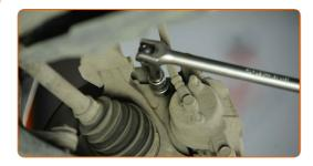
10 Remove the brake caliper.
