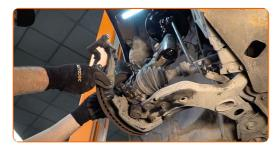
Remove the brake disc.
