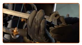
Clean the mounting seats of the tie rod end. Use a wire brush. Use WD-40 spray. 12
