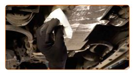
Screw in the new drainage plug and tighten it. Use a drive socket #21. Use a torque wrench. Tighten it to 34 Nm torque.
