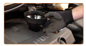
Pour oil into the engine through the filler. Required amount of oil: 4.5 L.
