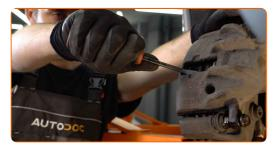
10 Remove the brake caliper.
