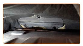
A Remove the cabin filter housing cover.
