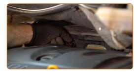
Remove the fender protection cover.
