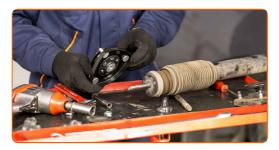
Tighten the shock absorber rod nut. Use a combination spanner #19. Use an adjustable wrench. Use a torque wrench. Tighten it to 25 Nm torque.
