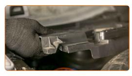
Remove the protective cap of the shock absorber mount. Use a flat screwdriver.
