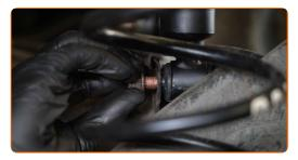
Tighten the lower fastener of the shock absorber. Use a combination spanner #21. Use a drive socket #21. Use a torque wrench. Tighten it to 127 Nm torque.
