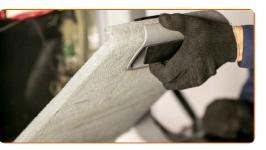
Tighten fixing bolts of the protective cover. Use a drive socket #10. Use a ratchet wrench.
