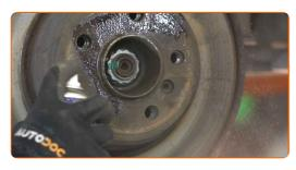
20 Unscrew the brake disc fastening. Use Torx T30. Use an impact screwdriver.
