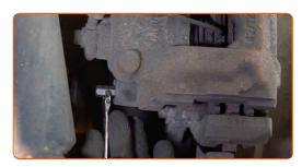
Detach the brake caliper retaining spring. Use a crowbar. Remove the brake caliper.
