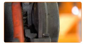
Unscrew the caliper bracket fastening. Use a drive socket #16. Use a tap wrench. Use a ratchet wrench.
