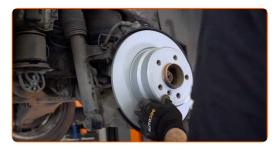
Tighten the brake disc fastening. Use Torx T30. Use a torque wrench. Tighten it to 16 Nm torque.
