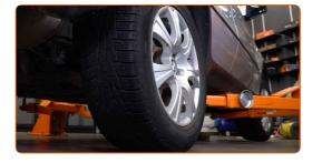
6 Loosen the wheel mounting bolts. Use wheel impact socket #19.
