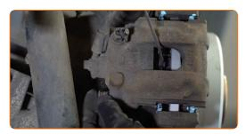
Install the brake caliper retaining spring.
