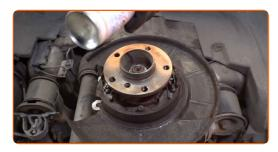
23 Install the brake disc.
