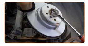
25 Install the brake caliper bracket.
