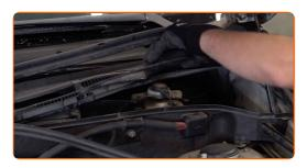
Unscrew the brake fluid reservoir cap.
