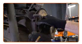
Remove the connector of the brake pad wear sensor. Use a crowbar.
