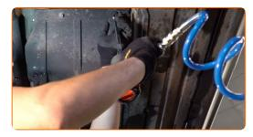
Unscrew the heat insulation fasteners. Use a drive socket #8. Use a ratchet wrench.
