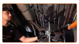
Unscrew fixing bolts of the protective cover. Use a drive socket #12.
