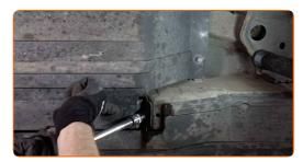
Screw in the heat insulation fasteners. Use a drive socket #8. Use a ratchet wrench.
