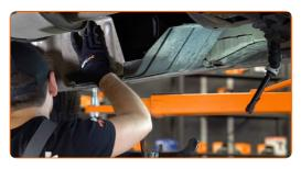
Tighten fixing bolts of the protective cover. Use a drive socket #12. Use a ratchet wrench.
