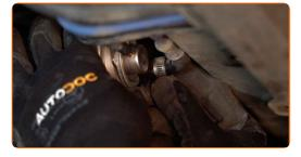
Tighten the fuel supply line fastening. Use a drive socket #7. Use a ratchet wrench.
