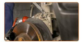
Remove the fastening bolt.
