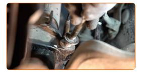
Disconnect the ABS sensor wiring.
