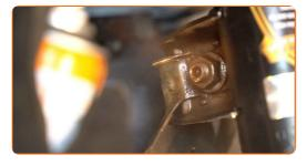
Fasten the brake hose on the strut.
