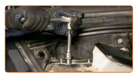
37.1 Install the windshield washer tank and tighten the bolts.
