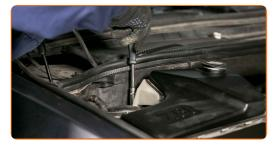
Remove the fender protection cover.
