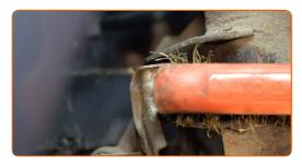
Unscrew the lower fastener connecting the shock strut to the steering knuckle. Use a combination spanner #22. Use a drive socket #22. Use a ratchet wrench.
