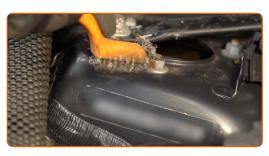
Unscrew the top fastening of the shock strut mount. Use a drive socket #13. Use a ratchet wrench.
